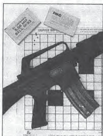
The Colt AR-15 can provide the hunter with better accuracy than he'd imagine, as this five-shot, 100 yard group is a little under two inches.
