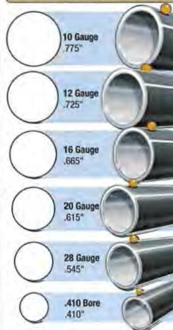
Sizes shown are the minimum inside bore diameter with a tolerance of +0.020". Data is presented courtesy of SAAMI.
