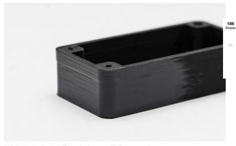
A black ABS print showing half coated with epoxy and half unprocessed
